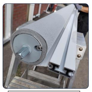
Inserting the Gearbox cap into the end of the blind
