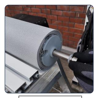
Inserting Idler pin and cap into the opposite end of the blind
